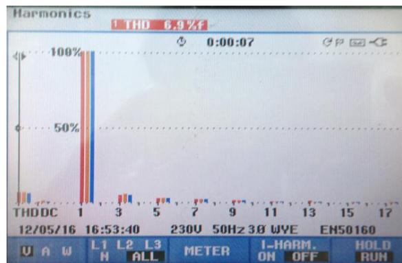
Fig 6.3 (c) Harmonic profile of  $V_{ph}$  by POD technique
